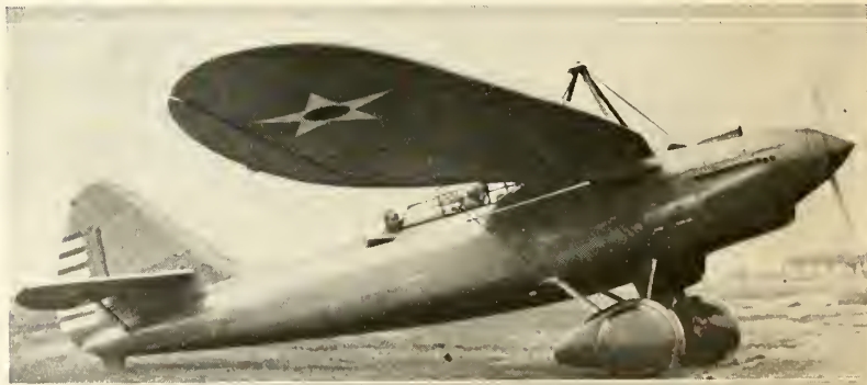
New Army Douglas observation plane, powered with 650-horsepower Conqueror engine
